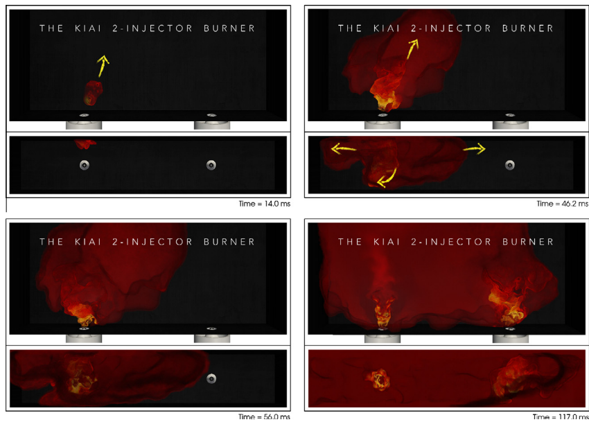
Fig. 18. LES results: instantaneous snapshots of the SP26 case ignition sequence visualized by the volume rendering of heat release (front and top views).
